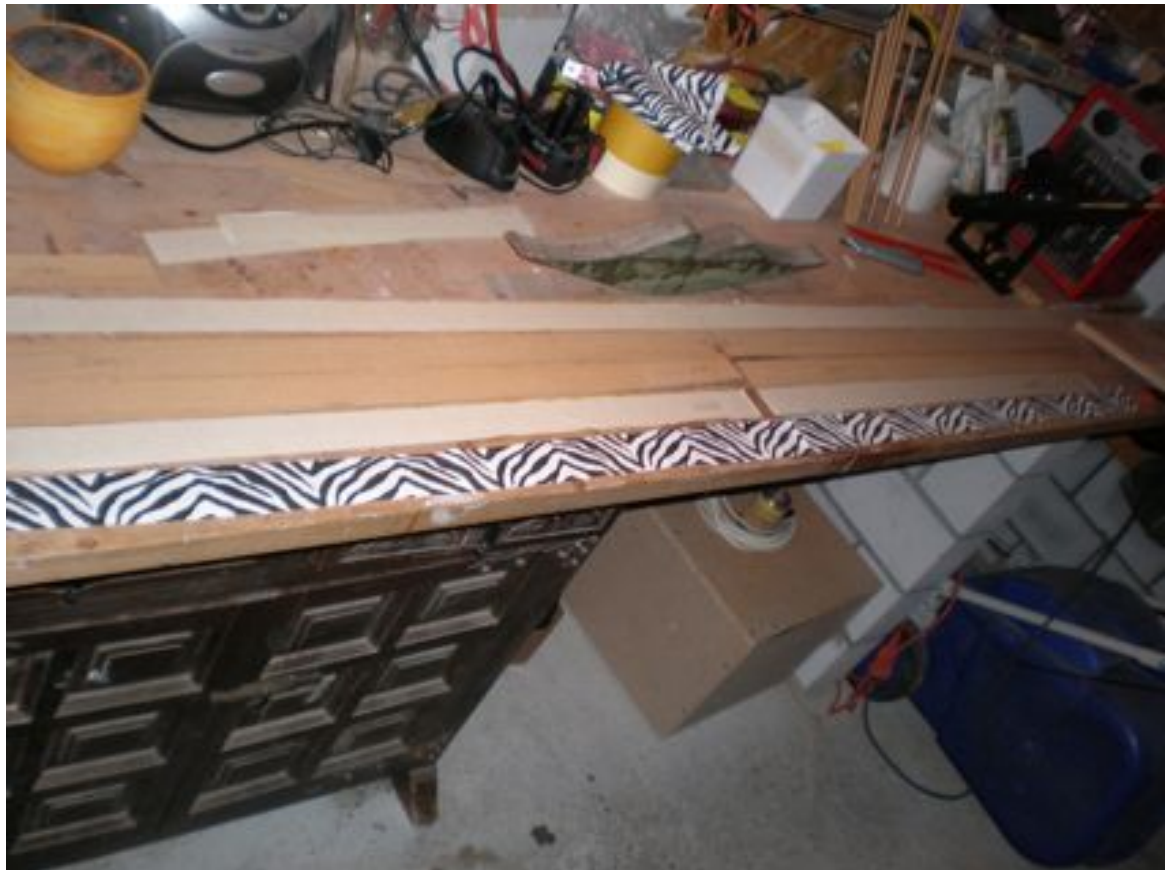
Picture 5: The lams, the glass and the camo strip ready for glue up
