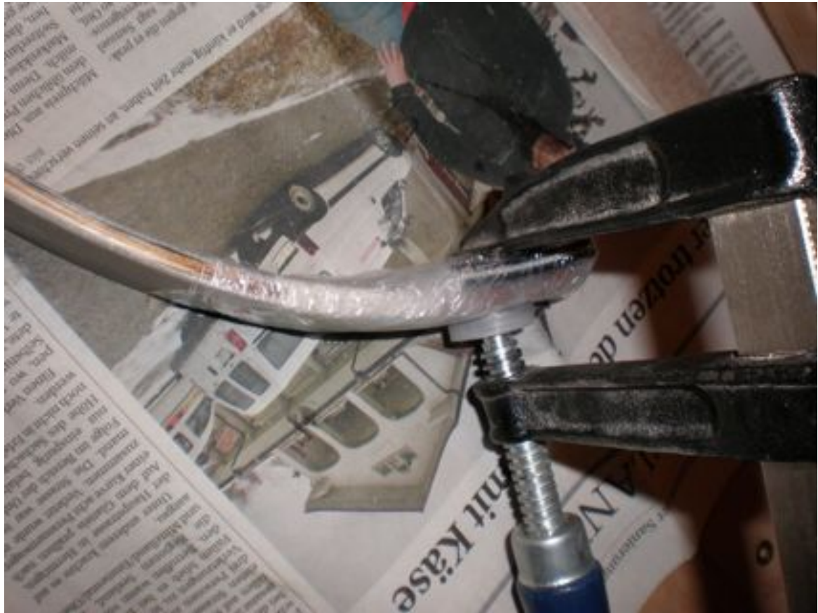
Picture 11: Glue up of the phenol tips
