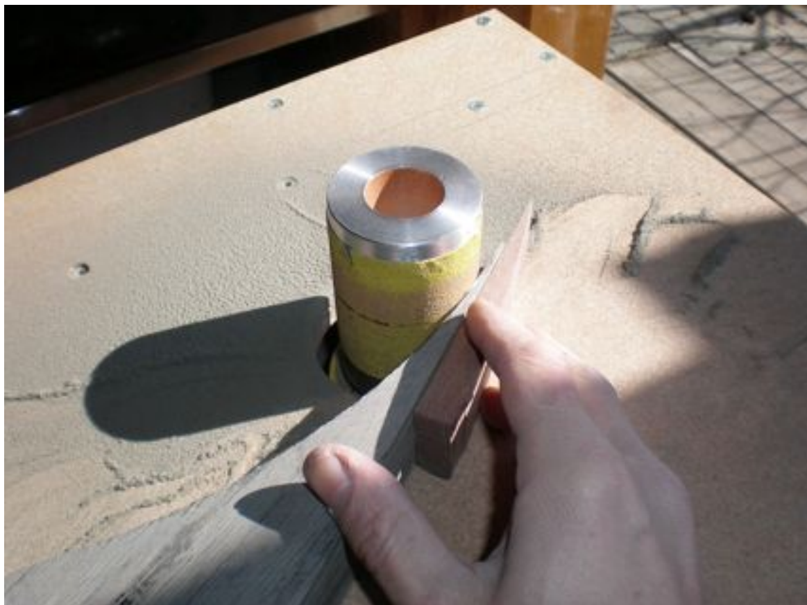
Picture 4: Sanding of the fades on the drum sander
