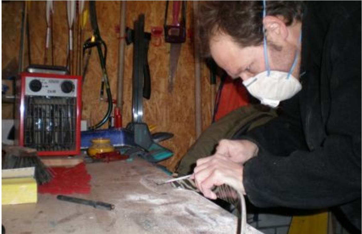
Picture 9: Filing of the string grooves
